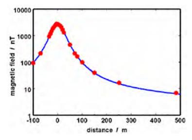
Figure 4-4. Typical Maximum Magnetic Fields from Different Voltage Power Lines, and Distance from Line
