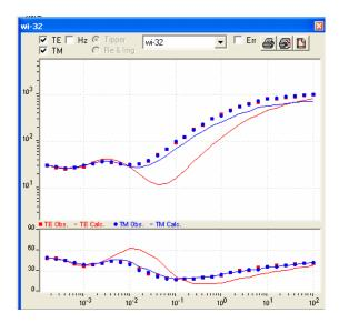
(c) Comparison of a 8 ohm-m Culebra vs. 0.1 ohm-m Culebra
