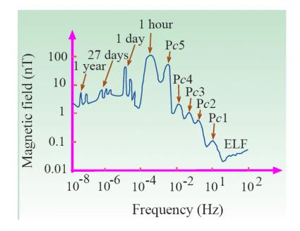
Figure 4-6. Typical Magnetic Spectra from MT Signal
