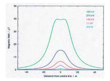
Figure 4-5. Magnetic Field Calculated by Distance from a 400 kV Power Line (Source: www.emfs.info/Source transmission.asp)
